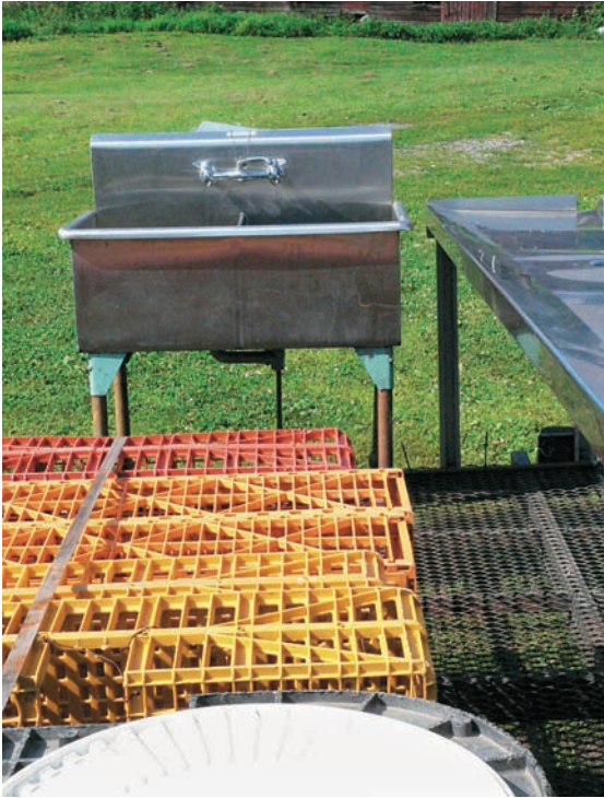
This stainless-steel double sink holds several birds for rinsing and initial chilling. Two people working the unit can process as many as 20 birds an hour.
